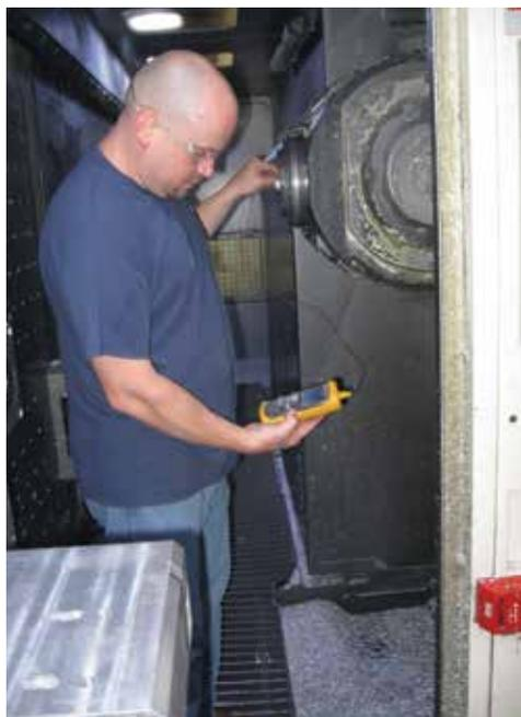
Spindle failures happen. The event is rare, but each occurrence formerly took the company by surprise and cost considerable time. How could the shop predict this failure? The answer proved to be the temperature inside the taper. An increase in temperature is the clue to order a spindle and schedule the replacement.
