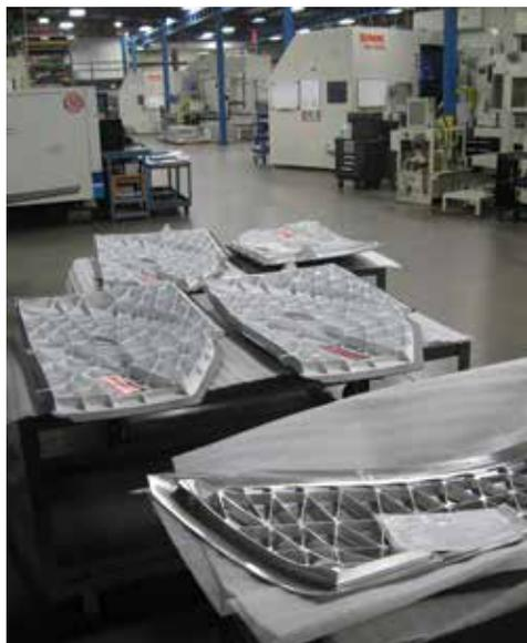
The sweet spot for Tech Manufacturing is aircraft components making extensive use of  $\frac{3}{4}$ -inch or 1-inch tools. The shop has fine-tuned its process and selected its machines specifically with that machining in mind. That said, the parts in the foreground do not fit this description—they make considerable use of smaller cutters. But the company machines enough of these parts that it was able to engineer a system to be competitive on these components as well.
