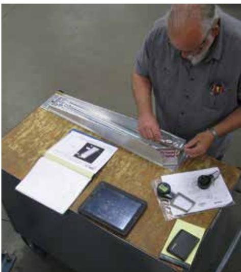
The shop has a quality area with sophisticated capability, but it's important to take care what work is sent here. One of the sources of unexpected delay discovered early on was the time spent carrying parts to and from inspection. The time-saving response to this has been to create gaging stations near the machines, such as the one at right.
