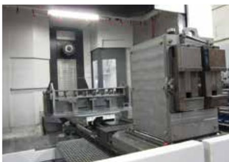
The pallet area outside the machine is open with ample crane access to streamline setups for shop personnel. It also features a large platform offering ample room for employees to safely maneuver around the pallet during setups. This platform also offered sufficient room for Park Industries to build a storage area for tools, gages and related devices operators commonly used when setting up new jobs.
