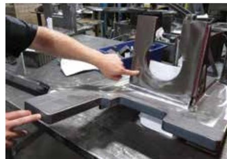
Here are a couple examples of spindle-reach issues that weldments present. The HN1000-S Bar machine's quill spindle offers 21 inches of W-axis motion to extend past obstructing features and enable the spindle to reach other areas of weldments that require milling or drilling.
